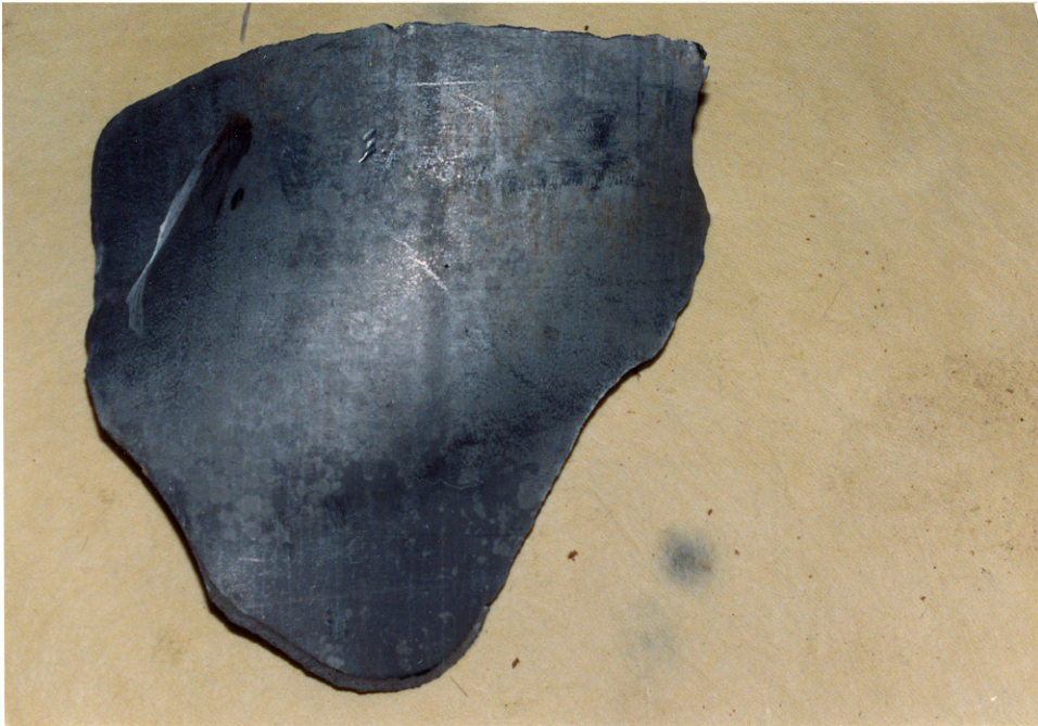
48. View of a fragment from the bottom left side of the aluminum CNG tank
